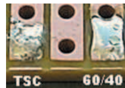
Fig.2. Comparing TSC lead-free solder to standard 60/40.
