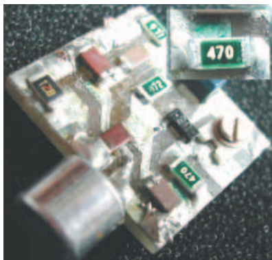
Fig.1. Use of SA (tin/silver) solder wire for a surface mount project.
