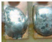
Fig.5. Lead contamination seen as a mottled surface.
