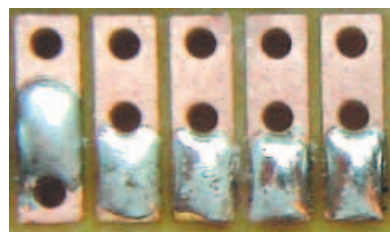
Fig.6. Effect of diminishing lead content.
